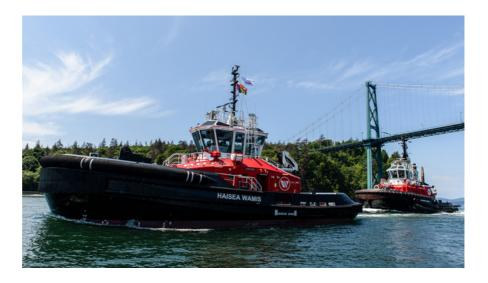
Once operational in Kitimat, HaiSea Wamis' substantial battery capacity (5,288 kWh) will enable a reduction of approximately 1700 tonnes of CO2 emissions per year compared to conventional diesel equivalent tugboats. Together with its sister vessels, HaiSea Wee'git and HaiSea Brave, the fleet of battery electric tugs is expected to save over 5,000 tonnes of CO2 emissions annually—equivalent to the emissions of about 1000 cars.
